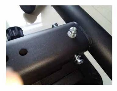
After inserting the stabilizer, use the screw to lock the tube tightly, and the other side is same operate like this one.
